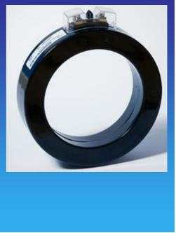
Description Current Transformers with a ratio of Ip/5, for measurement devices such as ammeters, kilowatt hour meters and multi meters. Ratios ranging from 600/5A to 3200/5A and a plastic case in accordance with Thermal Class E. Capable of being mounted using a busbar clamp the R113TW6 comes complete with sealable terminal cover.
